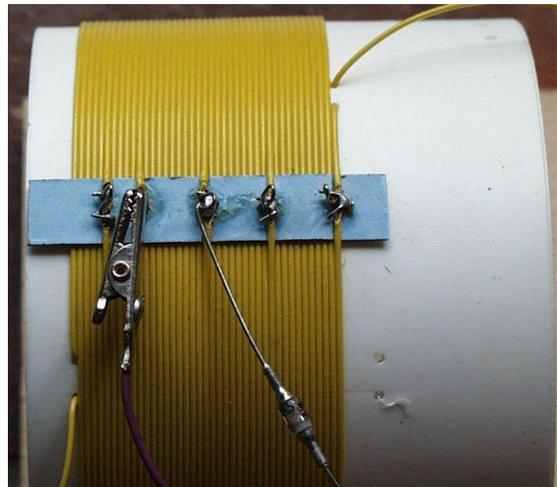
The best option, for maximum performance, is silver-plated Teflon-insulated hook-up wire if you have any in the junk box, but even common vinyl-insulated tinned stranded wire will work all right. Close-wound magnet wire is a bad bet, as eddy currents in the adjacent turns cause considerable loss.
