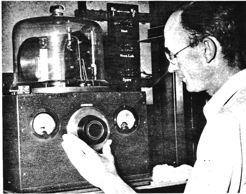
Master Frequency Standard of RCAC located at the Riverhead receiving station. Quartz crystal precision type oscillator with temperature, humidity and barometric controls.
