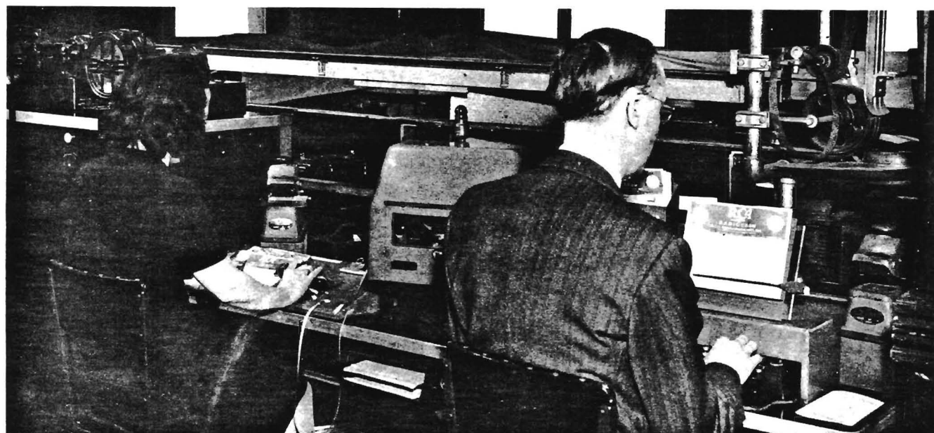
Radioprinter operating position in terminal operating office of R.C.A. Communications, New York City. Shows receiving and transmitting positions terminating one channel of an R.C.A. multichannel radioprinter circuit.
